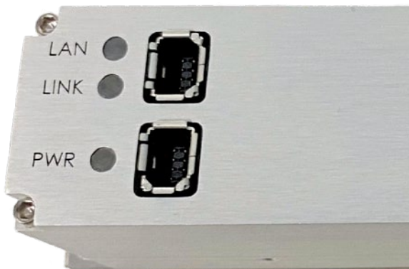
FIGURE 2-7: POWER & ETHERNET CONNECTIONS - EPX
